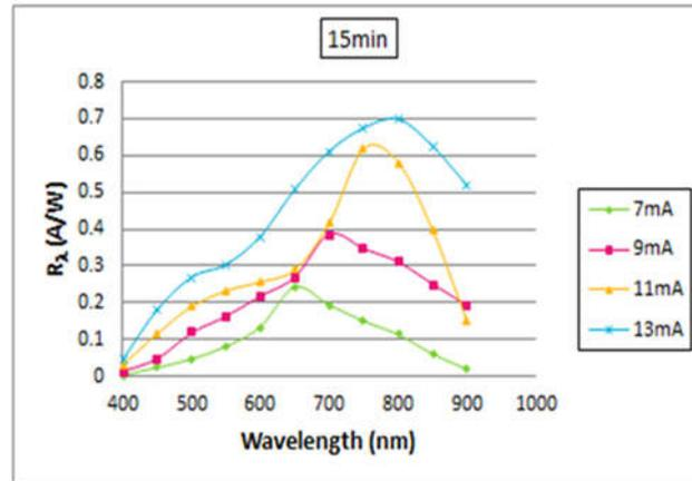
Figure (8): Responsivity  $R_\lambda$  as a function of various incident wavelengths for structure PS/p-Si HJ.
