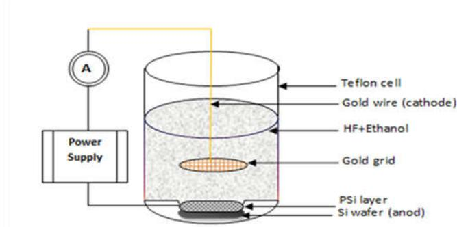
Figure (1): The set-up for preparation of PSi by using ECE process.
