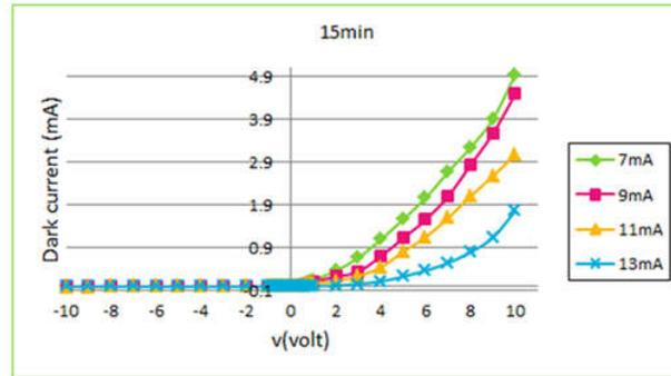
Figure (3): The Current -Voltage characteristics of PSi prepared with different etching current .
