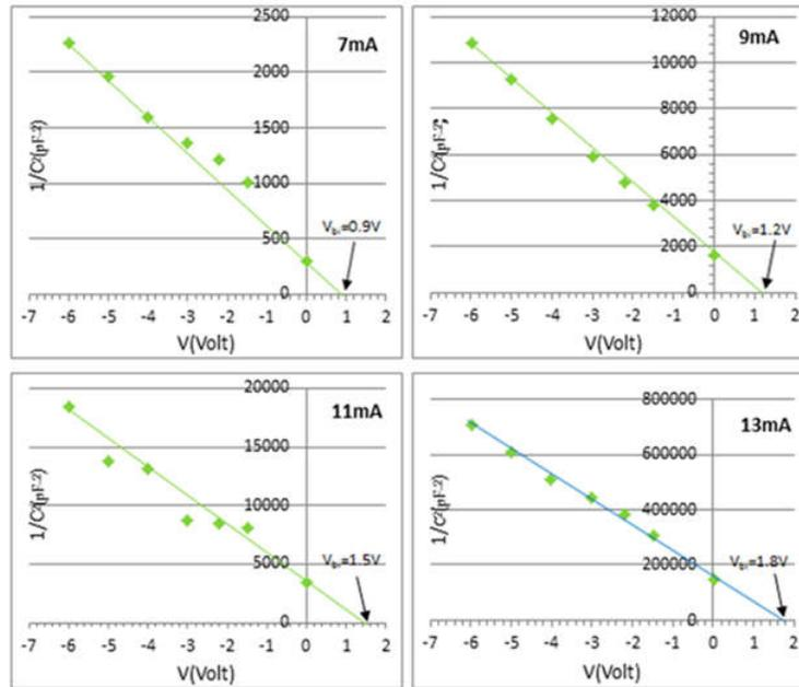
Figure (7): The inverse capacitance squared versus Voltage
