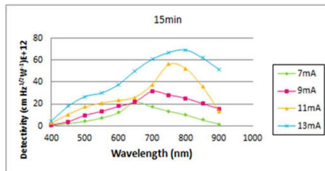
Figure (9): Measured detectivity of the Al/ PS/p-Si/Al photodetector versus wavelength of incident light.
