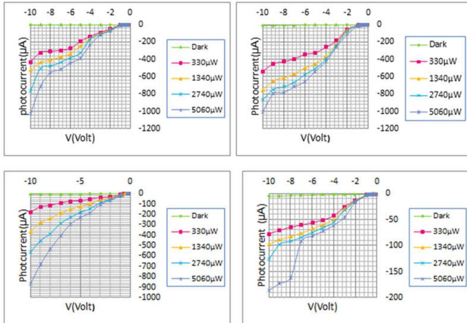
Figure (5): The Photocurrent Density as a function of the applied reverse voltage for Al/PSi/p-Si/Al.
