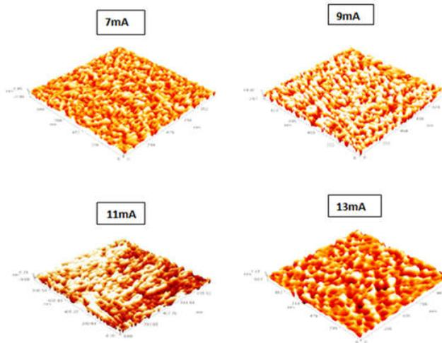
Figure (2): 3D AFM images of p-PSi surface (at 15min and different etching currents)
