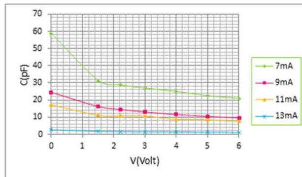
Figure (6): (C-V) characteristics of PSi
